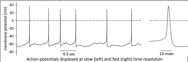
Recording Action potentials requires an electrical connection to the inside of the cell, which is achieved using a glass electrode, basically a hollow glass tube that has been heated and drawn down to a fine tip. The tube is filled with a salt solution that is compatible with the inside of the
